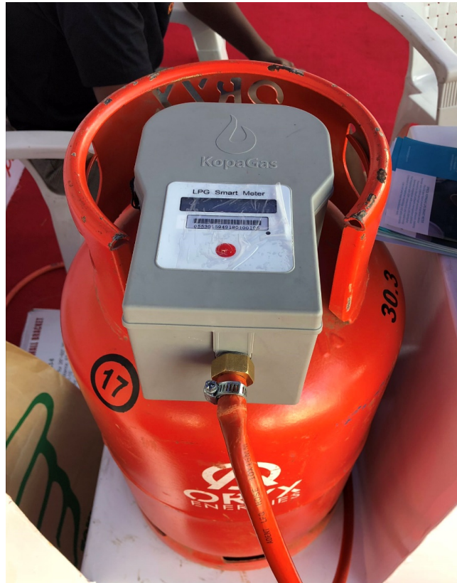
Figure 1. LPG smart-metre fixed to the gas cylinder. Photo by: Ndunguru, 2019.
