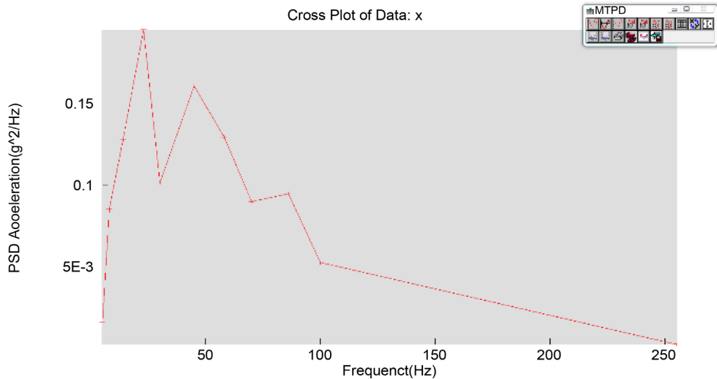
Figure 12. X direction amplitude frequency excitation curve test bench.
