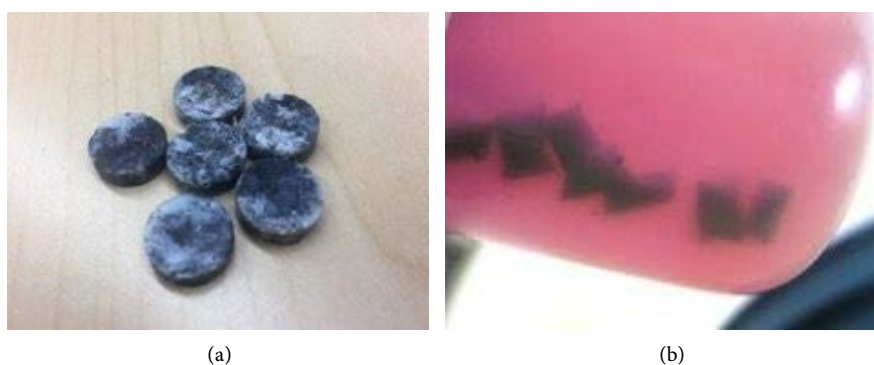
Figure 2. (a) Pellets with \text{KMnO}_4 encapsulated in PCL; (b) Pellets release \text{KMnO}_4 in water.
