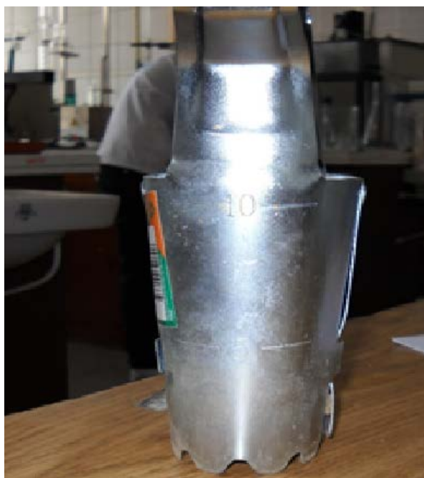
Figure 1. Soil sampling device (device made by author).
