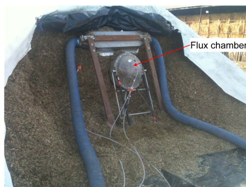
Figure 1. Flux chamber covering the surface of an Ag-Bag silage face for air sampling.
