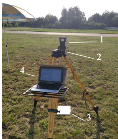
Figure 3. Device for diffuse plate spectra registration: 1—SSP-600 spectrometer; 2—a tripod with a bracket; 3—diffuse plate; 4—laptop computer.
