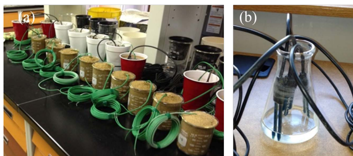
Figure 2. The (a) Watermark and (b) EC-5 sensors calibration procedure in the laboratory.
