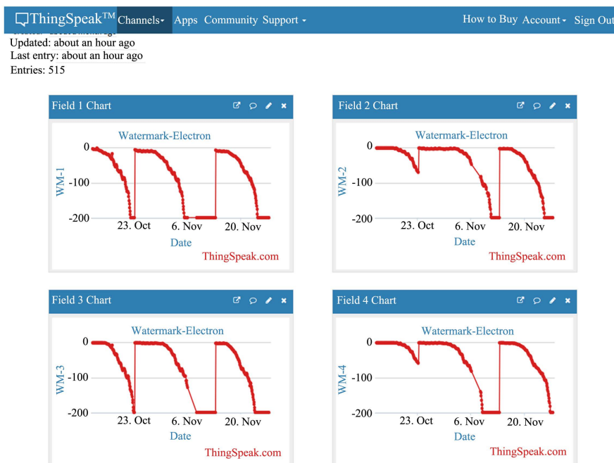
Figure 8. The Volumetric Water Content (VWC) of soil collected during 3 drying cycles in the laboratory using four Watermark sensors.
