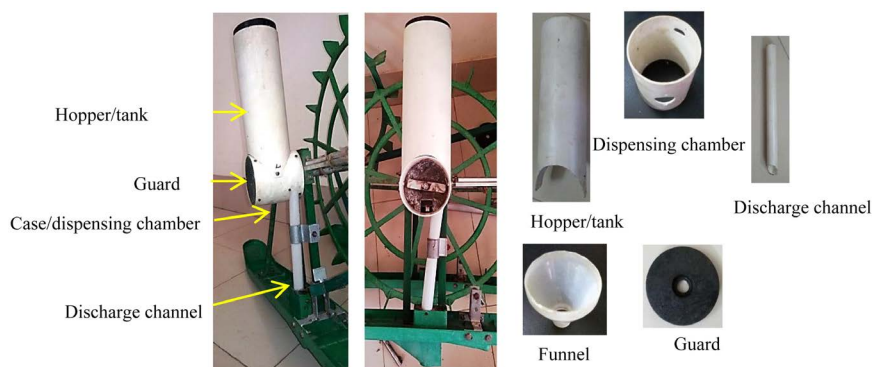
Figure 7. Photographic view of the hopper, funnel, dispensing chamber, guard and discharge channel.
