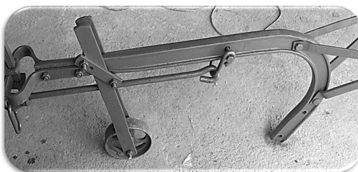
Figure 1. Standard ox-plough beam with bottom detached.
