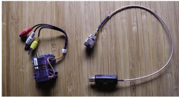
Figure 9. A low-cost antenna alignment set: a signal generator (video sender) and a low-cost spectrum analyzer.
