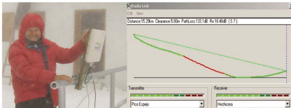
Figure 10. The 5.8 GHz wireless bridge between Pico Espejo (4765 m) and Merida.
