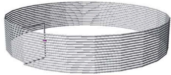
Figure 3. A depiction of the 15-turn air-core loop modeled in NEC. The loop had a diameter of 5.08 cm and an overall length of 1 cm.
