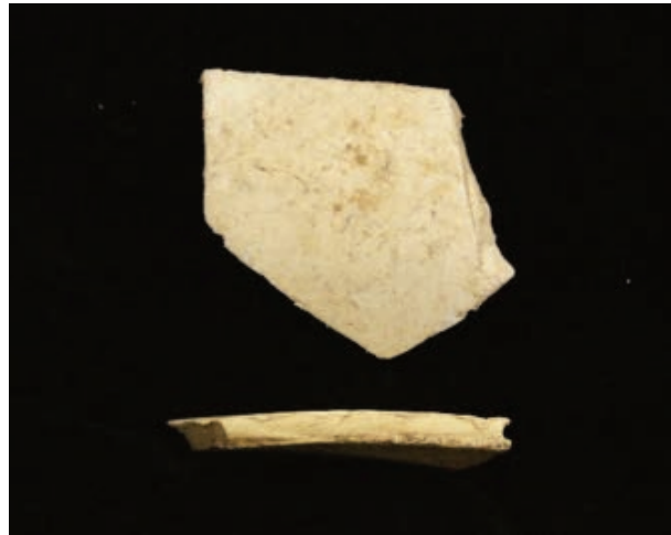
Figure 15.5 Fragments of plastic PVC pipe, such as those seen in this photo, may be mistaken for human bone.
