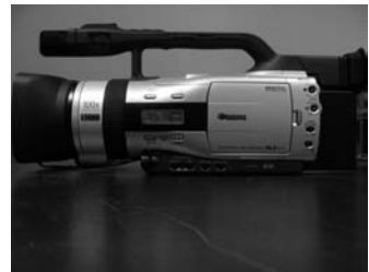
An example of a 3CCD camera, the Canon GL-2.
