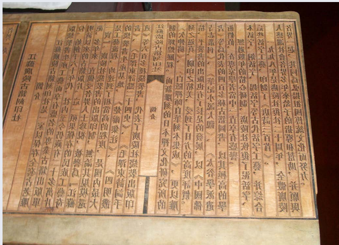
Figure 4.23 | A woodblock used to print one page of classical Chinese | The characters read from top to bottom and right to left. During the Song, individual, moveable woodblocks with one character were also carved and arranged in square frames.
